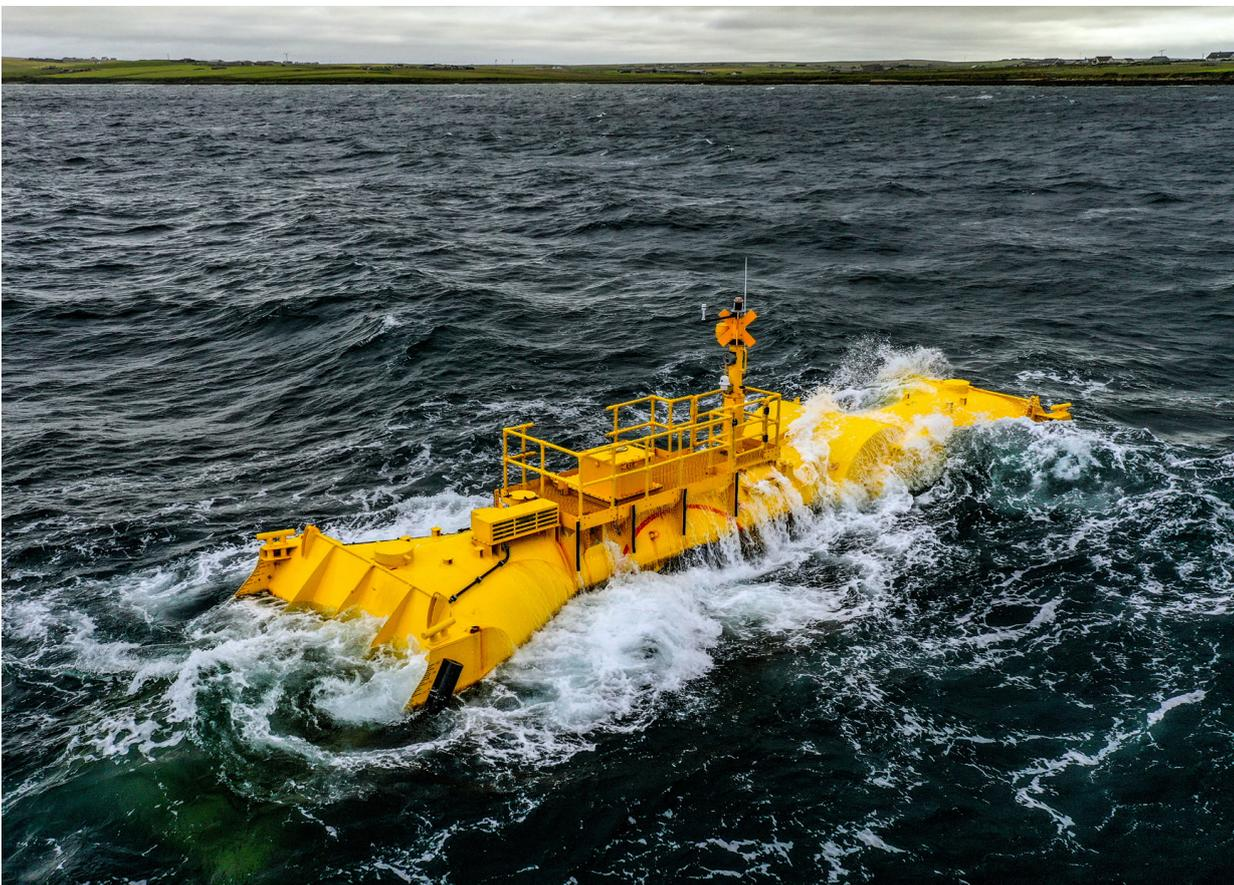
There are dozens of wave energy sites worldwide, demonstrating machines from 1kW up to tens of MW in scale. Just as the UK is at the forefront of offshore wind energy, many of these are hosted at UK testing facilities (see map). For example, Orkney hosts the European Marine Energy Centre (EMEC) which is a test bed for multiple technologies from UK and European manufacturers.
